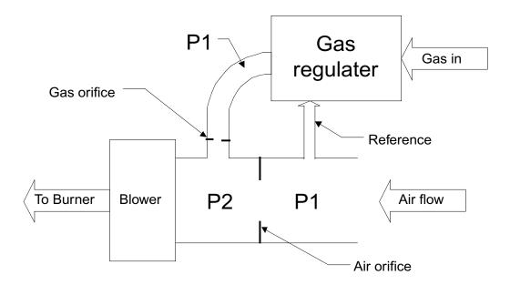
Referring to the sketch above, the Gas regulator is a precision device that detects the pressure, P1 that exists at the air inlet orifice via a reference connection and creates the same pressure ahead of the gas orifice. The pressure P2 is the same for both orifices. Thus:  $\Delta P(gas) = \Delta P(air)$
